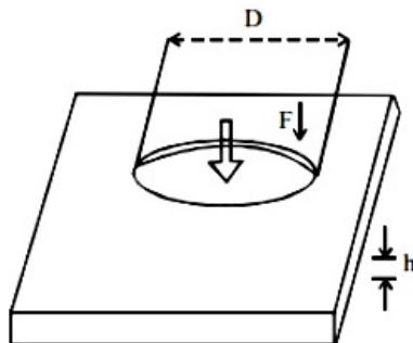
Shearing strain is created along the side surface of the punched disk. Note that the forces exerted on the disk are exerted along the circumference of the disk, and the total force exerted on its center only.
